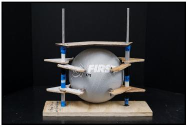
Wooden prototype of pneumatically actuated fingers
