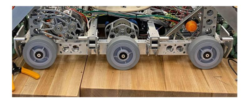
The Drivetrain is a six wheel West Coast Drive that is designed for simplicity and robustness. We chose colson wheels because we wanted to have low maintenance but to still have good performance. Additionally, the gear ratio of the drivetrain was designed for fast acceleration for shorter distances and overcoming defense.
