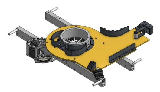
The turret is designed to quickly and reliably turn the catapult, flippy arms, and climber, which are all mounted on top of the turret.
