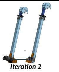
• Double spools, powered by a versa gearbox connected by a main shaft, no friction brake assembly instead 1:100 gear ratio
