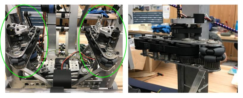
The Flippy Arms were designed to transfer the cargo from the intake into the Catapult. They hold the cargo in place in the catapult as the turret aligns and then open up to release the ball when the catapult fires.
