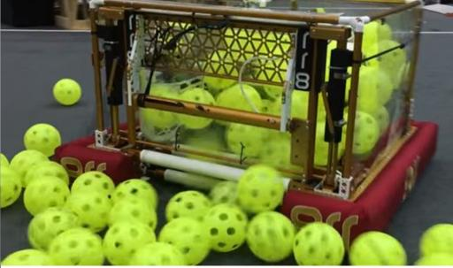
One Banebots 775 4:1 gear reduction 1:1 pulley 1.75" roller
