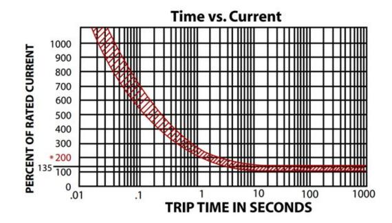
150 % overload = 3.9 - 47 seconds 175 % overload = 2.2 - 9.2 second \* 200 % overload = 1.5 - 3.9 seconds 250 % overload = 0.8 - 1.8 seconds 300 % overload = 0.5 - 1.1 seconds 400 % overload = 0.3 - 0.6 seconds 500 % overload = 0.2 - 0.3 seconds
