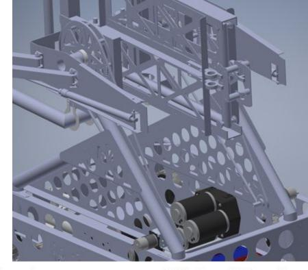
Two RS 775 motors 100:1 VP gearbox 100:22 chain reduction
