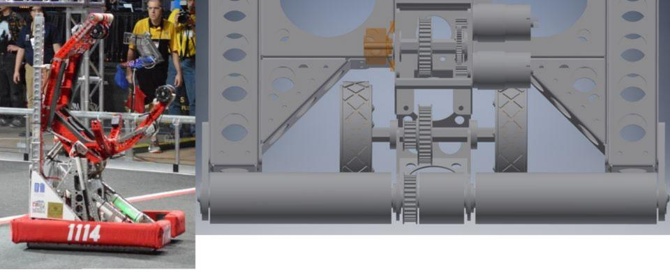
Two RS-550 motors 4:1 gearbox reduction 30:18 pulley reduction 2" roller
