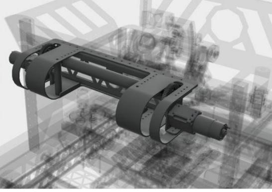
2 775pros 25:1 VP reduction 54:16 Gear reduction 1.25" winch
